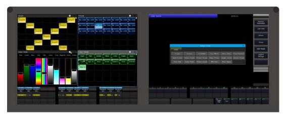
The operating menu is on the right side of the right touch screen. Most of the operations are worked on the touch screen. Different working windows can be selected and displayed on both touch screens according to the control needed.
